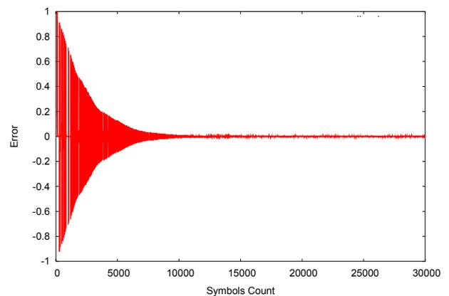
Fig9: Equalization with reduced no. Of taps
