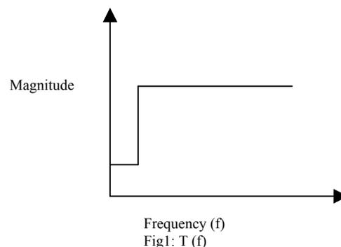
When allowed to equalize the Channel having spectral nulls, the equalizer would introduce a very high gain wherever there were spectral nulls. To learn these spectral nulls the equalizer is taxed in time, computation and structure.
