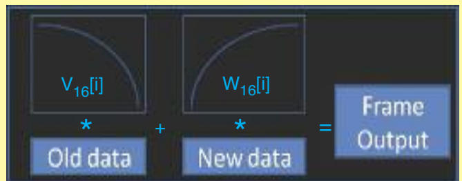
Figure 4: Diagram of Window Overlap Add module
