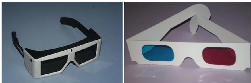
Figure 2 LCD shutter glasses and Paper anaglyph filters
