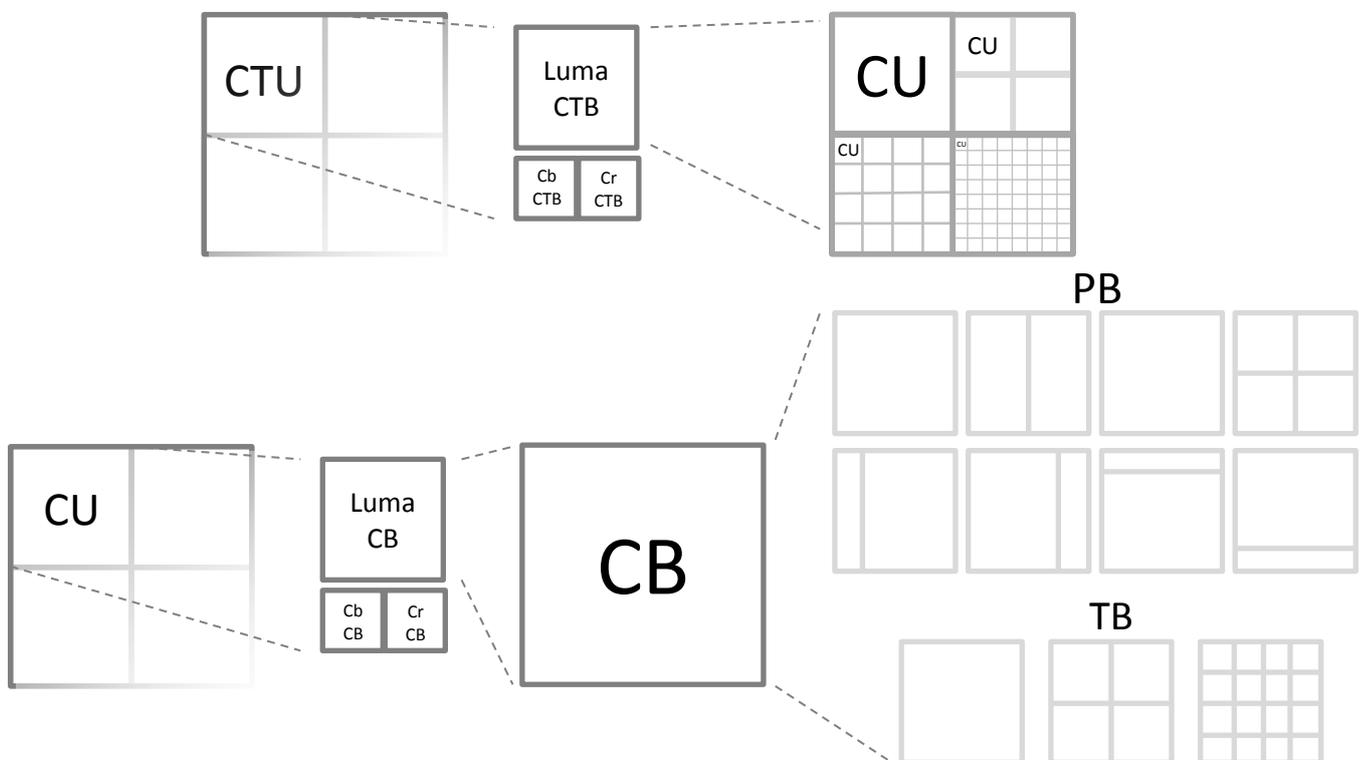
Figure-1: Coding trees and blocks in HEVC (CTU: Coding Tree Unit, CU: Coding Unit, CB: Coding Block, PB: Prediction Block, TB: Transform Block)
