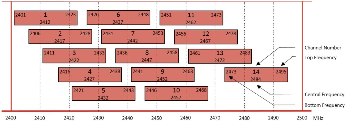
Figure 1 - 2.4GHz Channels and Frequency Spectrum
