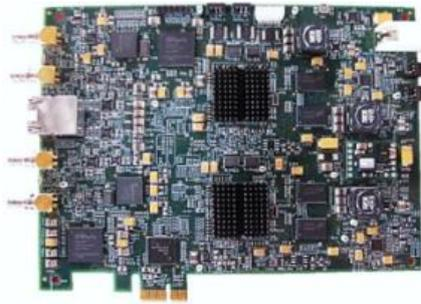
Frame Grabber is a term typically used to refer to devices that provide audio/video capture functionality on personal computers (PC). Frame grabbers come with a variety of forms and features such as PCI capture cards, USB webcams, FireWire cameras to name a few. Some frame grabbers capture analog only / digital only signals while some may support both. The selection of the right type of frame grabber is entirely dependent on the end use-case.
